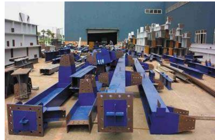
Fabrication of Steel Structures
